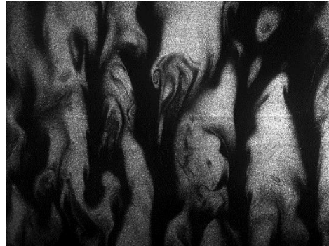
Horizontal plane PIV image from z = 3.5 mm at Ri = 2.0
