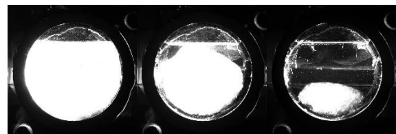
Development of the melt front in a circular enclosure heated from the walls, 5 degrees above melting. The white region is unmelted PCM. (Left – 30 minutes, centre – 135 minutes, right – 225 minutes)
