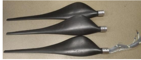
Carbon fiber blades ready to install on the turbine. Note that only one of the three blades is instrumented.
