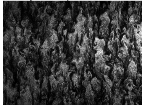
Horizontal plane PIV image from z = 3.5 mm at Ri = 0.1
