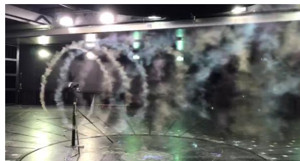
Smoke visualization of the wake
