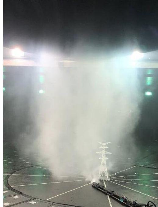
Full aero-elastic transmission tower model under a simulated tornado conducted in WindEEE research institute
